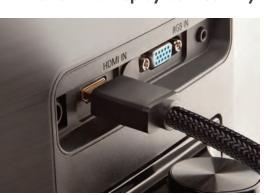
The Chromebit plugs directly into a display's HDMI port, or alternatively connects via included HDMI extension cable for tight connection locations.
